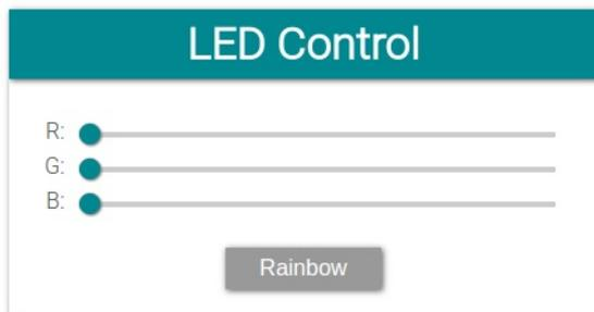
Use the sliders to adjust the color levels of the LED, and press the Rainbow button to enable the rainbow effect.
